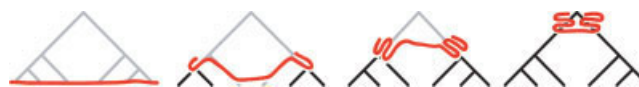
Fig. 1. Trees describe folding routes. Horizontal treecuts describe the state of the chain at any point in time. [Color figure can be viewed in the online issue, which is available at www.interscience.wiley.com .]
